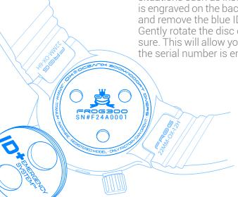
The blue ID+SYS™ disc screws on and off effortlessly. Simply place your fingers on it and rotate without applying pressure to remove or reattach it. There's no need to overtighten—just a few turns will suffice.
