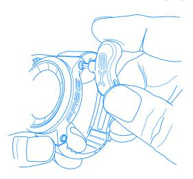
Switching straps is easy with the Allen tool:
